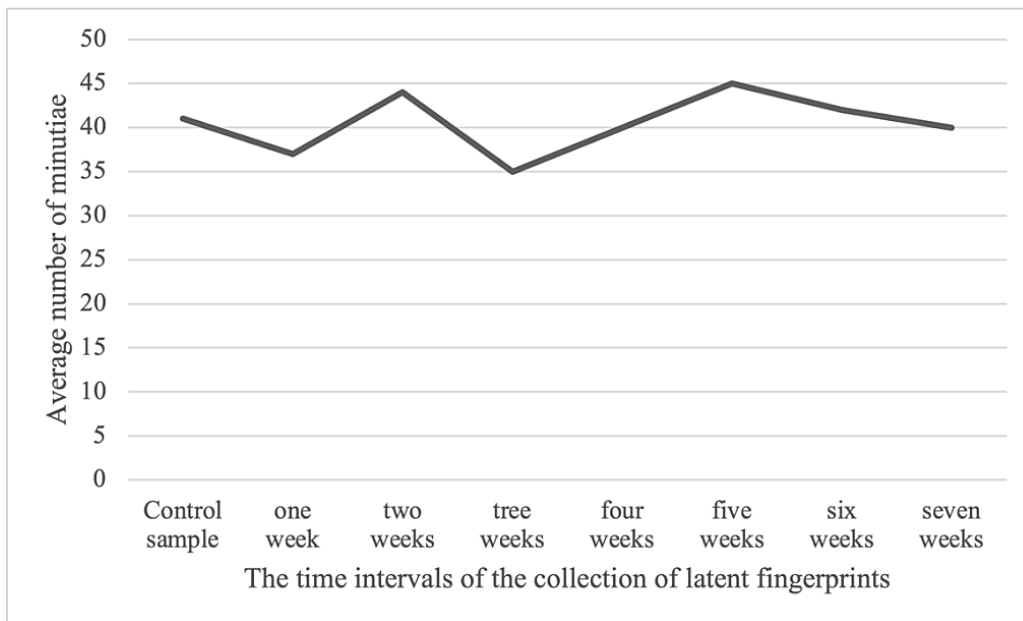
Fig. 3: Graphical representation of the average number of minutiae on degraded latent fingerprints due to direct sunlight at different time intervals
